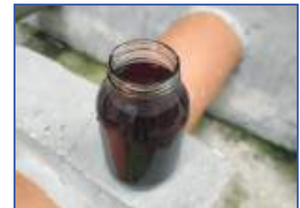
Figure 3b: Raw sewage contaminated by remnants of partially degraded coloured dyes from trade effluent discharged by factories.
