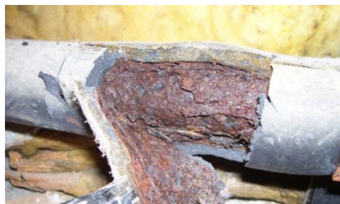
Corrosion under insulation on a piping. Courtesy: https://www.russelltech.com/News/ArtMID/719/ArticleID/255/Mitigating-The-Risks-Of-Corrosion-Under-Insulation-With-Russell-NDE-Systems
