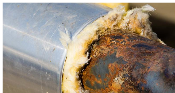
Corrosion under insulation found on pipe Courtesy: https://conceptgroupplc.com/glossary/what-is-corrosion-under-insulation/
