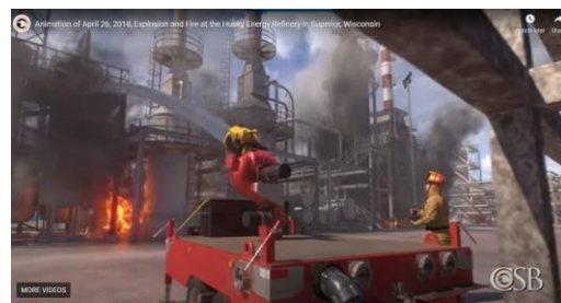
Large fire monitors designed to deliver adequate fire water, deployed in the right location are essential to prevent spread of a fire [Ref. 3]
